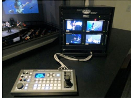
The Vaddio Precision Camera Controller works in conjunction with the FOR-A HVS-300HS portable video switcher for joystick and CCU control. Vaddio PreVIEW Rack Mount Monitors are also being used to monitor Preview and Program outputs. “Vaddio’s price point and ease of functionality were a good fit for Parkway’s needs,” explained Smits. “They are also easy to install and intuitive to operate.”
